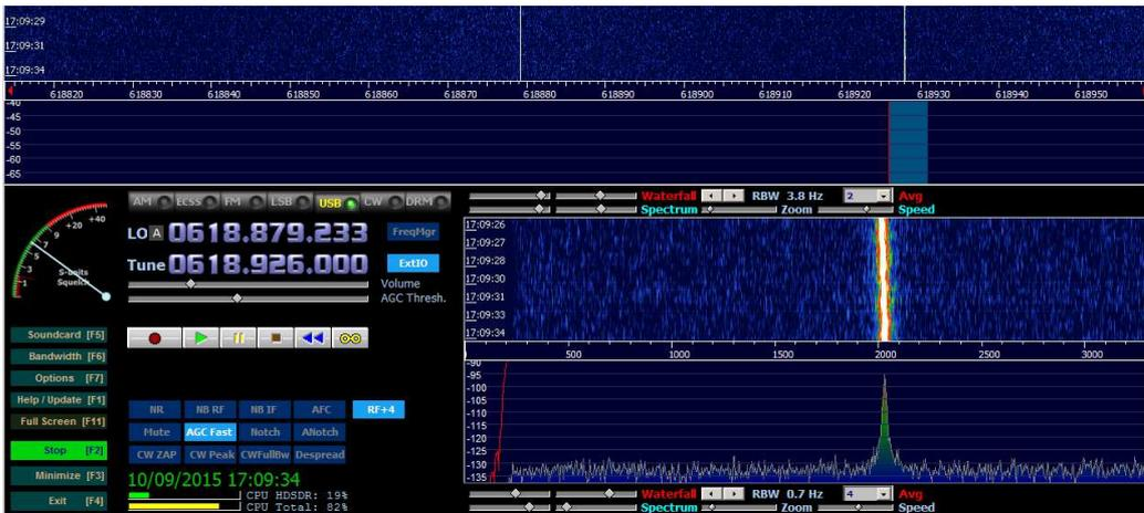
And then the same signal when the external 27Mhz reference is used
