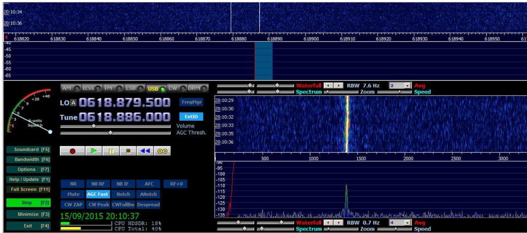
Added phasenoise due to the 27MHz PLL is really minimum. You can hardly notice by ear a significant difference when using the LNB crystal or the external reference
