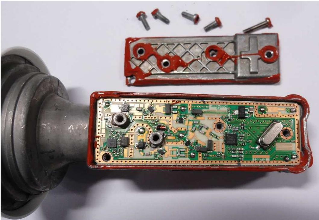
On the right side there is clearly the 27Mhz crystal and the two IF outputs. We will keep the main output as IF which is located down on the right side. The other output (up on right side) will be modified to inject our 27Mhz disciplined reference. First step is cutting the track of this secondary IF output
