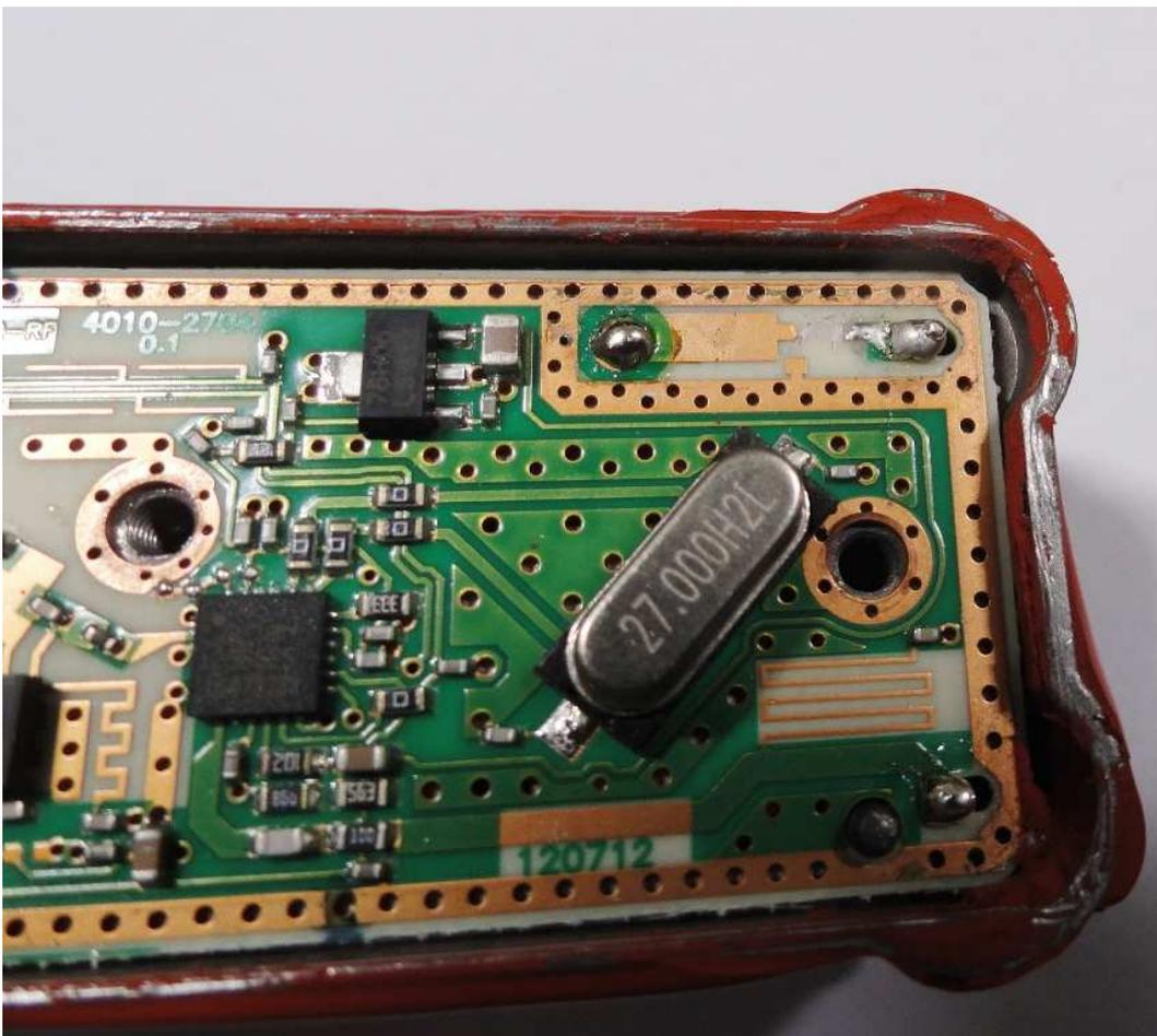
At this point we install an small SMD 0603 1nF ceramic capacitor which will be in serial with the signal to block any incoming DC. The other side of capacitor will link to the closest pin of the quartz crystal using an small wrapping wire
